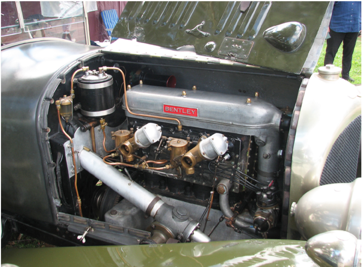
Above: Ian & Tina Oliver presented their two Bentley 'Speed' models which are 100 years apart. This is their 1924 3-Litre with, below , its magnificent engine. Note the characteristic S.U. 'sloper' carburettors. See also opposite page, top .
